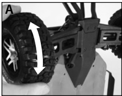
A Rotate the rear wheels slowly until the output shaft keys into place.
